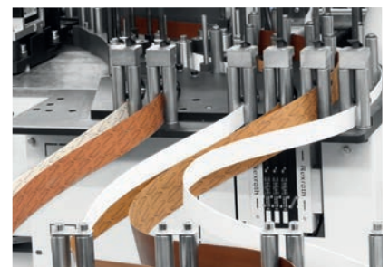
Six-coil magazine Automatic infeed of 6 different edges.
