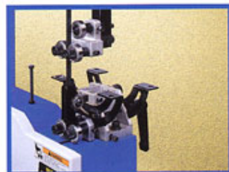
Upper and lower ball bearing blade guide system
