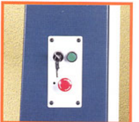
On/off push button with safety key lock
