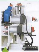
Sizing System S Top and bottom saw construction may effectively avoid tearing problems when cutting laminated panels. Scoring and main sawblades are closely positioned to facilitate adjustment.
