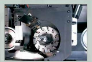
STRAIGHT AND PROFILED KNIFE SHARPENING DEVICE (OPTIONAL)
