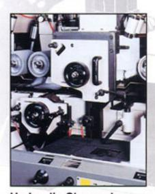
Hydraulic Clamped Outboard Bearing System (Optional)
