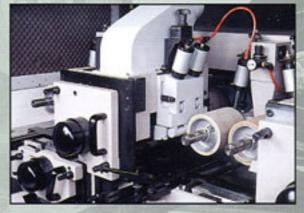
Pneumatic Cylinder for Chipbreaker on Top Spindle
