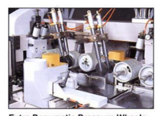
Extra Pneumatic Pressure Wheels for Vertical Spindle (Optional)
