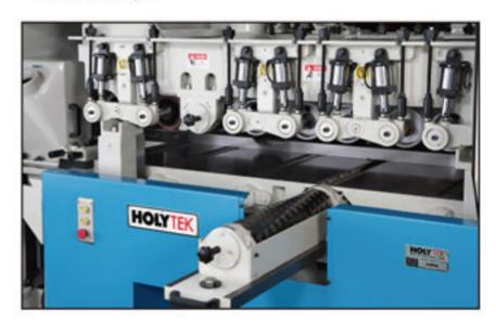
Heavy-duty Spiral Cutterhead for Bottom Spindle
