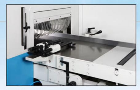
Infeed Unit and Precision Guide Fence with Table Rollers and Side Pressure Roller Allow Smooth Feeding.
