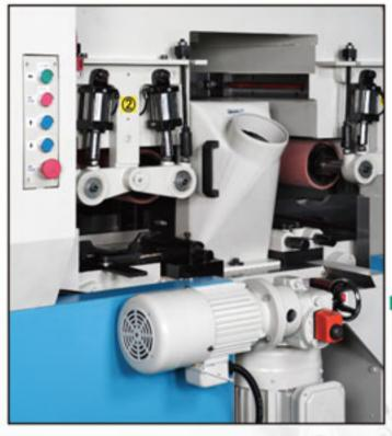
Vertical Spindle Unit and Digital Readout Setting by Motorized Moving.
