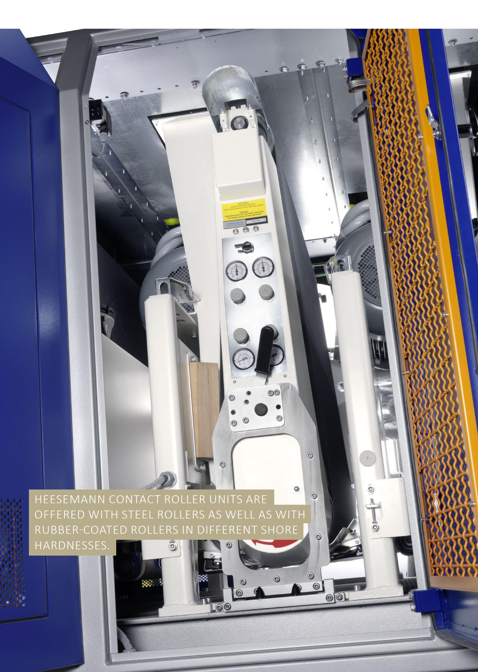
HEESEMANN CONTACT ROLLER UNITS ARE OFFERED WITH STEEL ROLLERS AS WELL AS WITH RUBBER-COATED ROLLERS IN DIFFERENT SHORE HARDNESSES.
