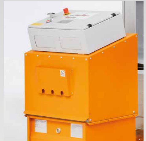
Control cabinet of a Compacto briquetting press
