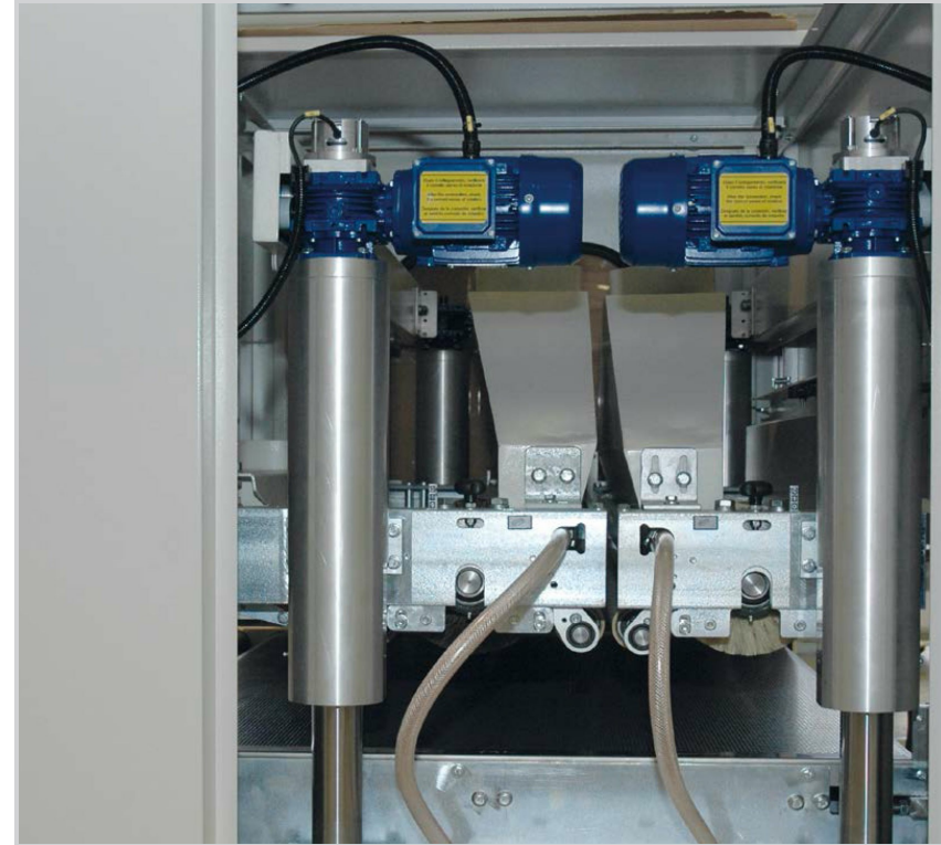
SOLUTIONS FOR CLEANING FLAT AND SHAPED PANELS, EDGES INCLUDED, WITH BRUSH/AND, BLOWERS AND DEIONISING BAR
