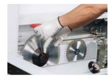
This easy-to-use, fast clamping system speeds up blade changes on both main and scoring saw.
