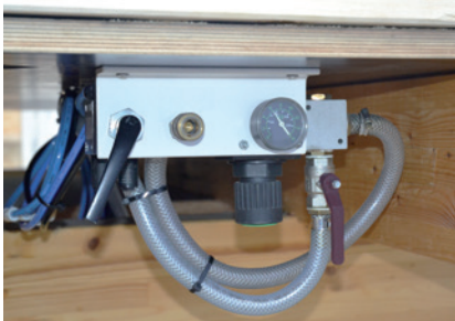
Includes pneumatics systems for the central air supply and controlling the C-PowerTec clamping beams
