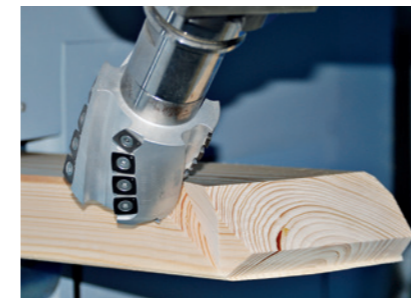
Producing a tenon joint
