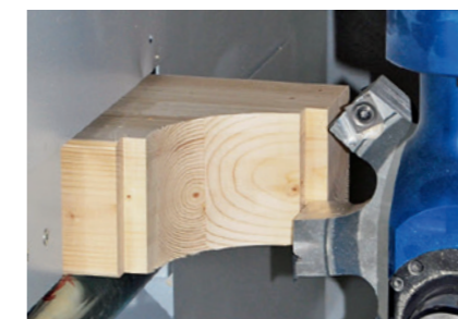
Machining the rafter head
