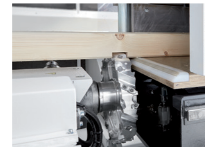
Production of a notch with the routing unit
