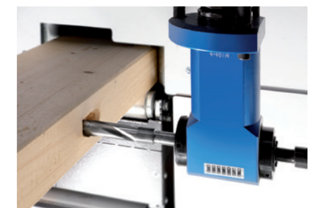
Production of mortises and pockets
