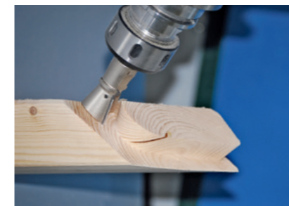
Dovetail at the jack rafter
