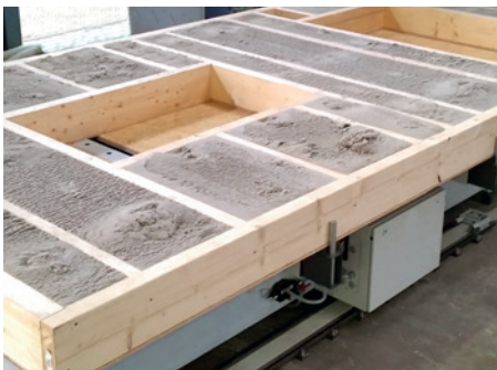
Wide range of insulation materials , such as cellulose, wood fiber, mineral wool can be insulated.
