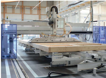
Fully automated positioning of the insulation plate above the respective frame work compartment.
