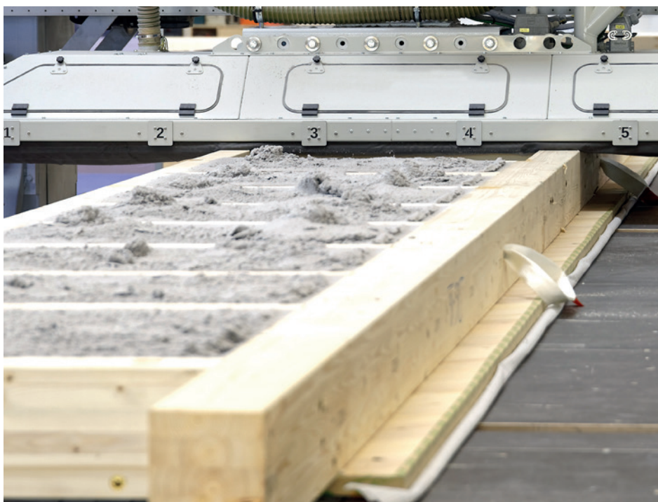
Automatic calculation of the filling quantity enables the optimal and consistent density distribution of the insulation material in each compartment.
