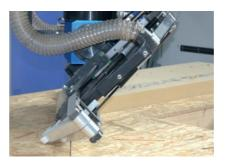
Sawing unit with a built-in protective cover and suction hood
