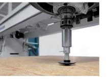
Marking and labeling Marking of panel joints, slat positions, or shuttering boards enables fast and easy
