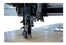
Chuck for a second fastening unit Different fastening units enable the attachment of various types of sheathing material.
