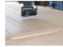
Gluina Using a multi-nozzle system means that individual components and surfaces can be glued quickly.
