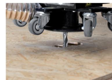
Interpolating routing processing
