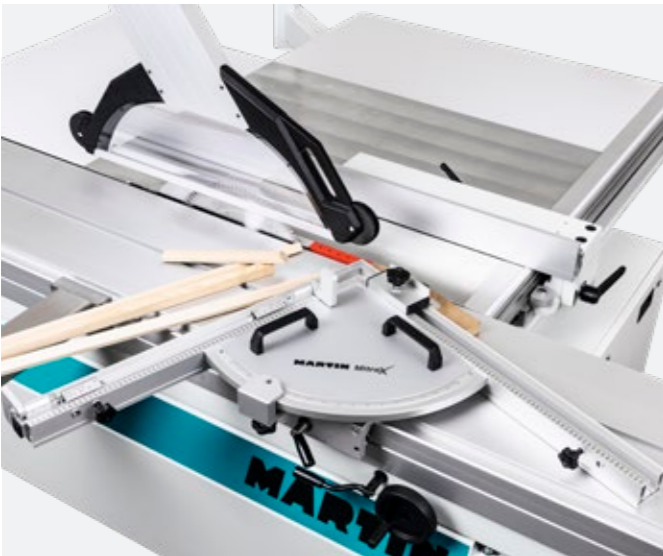
MitreX with analogue angle display | Txx79/1
