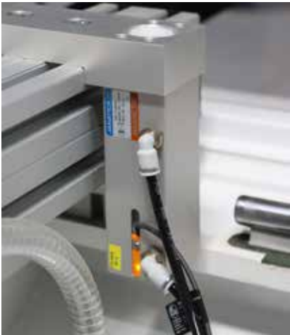
Electronic cylinder surveillance Enhanced security with the electronic surveillance of lower cylinder positions at all integrated stops
