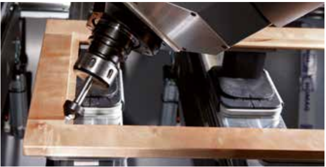
Square corner routing for a glass rebate
