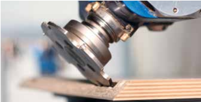
Cutting recesses for connecting fittings
