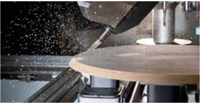
Chamfer trimming on a table top
